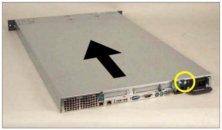
Figure 25: Installing the cover
